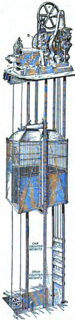
Fig. 50. Overhead type elevator machine,
